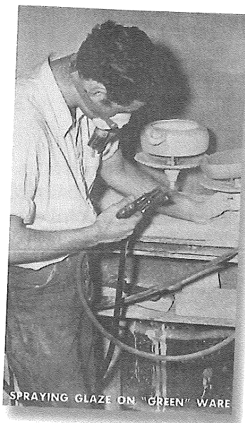
Standard size, B&W. (a) Caster pouring slip, dumping slip, and removing ware from molds; (b) glazer glazing a 94V and a 205; (c) loading the tunnel kiln at one end; and (d) unloading finished ware at other end of kiln.
